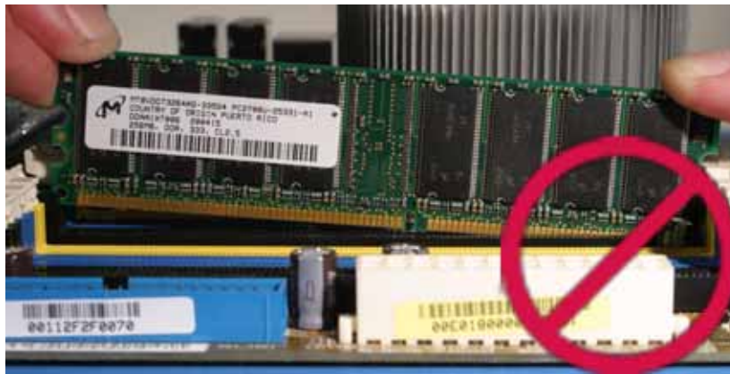
Figure 30: Never Insert the Memory Module by Pushing on One Side Only
