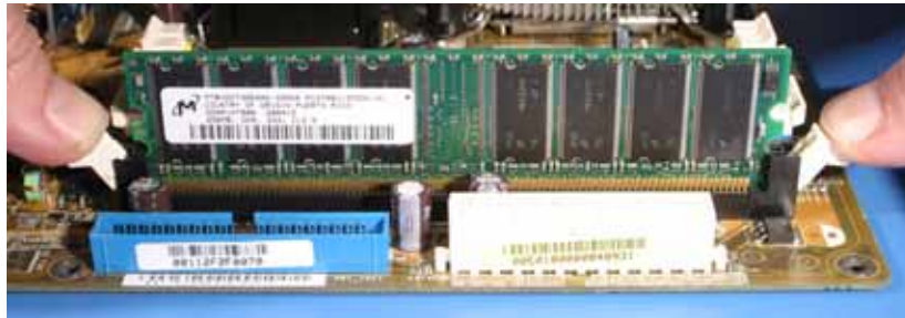
Figure 37: Remove the Module, Touching Only the Edges of the PCB
