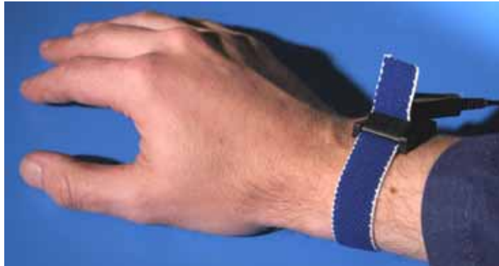
Figure 2: Always Wear ESD Straps When Inserting Modules into Sockets
