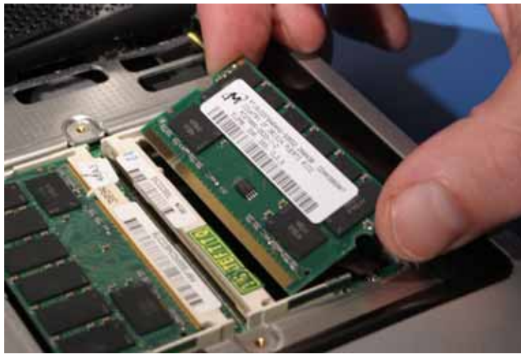
Figure 16: If the Module Cannot Be Inserted Easily, Remove It from the Socket and Start Over
