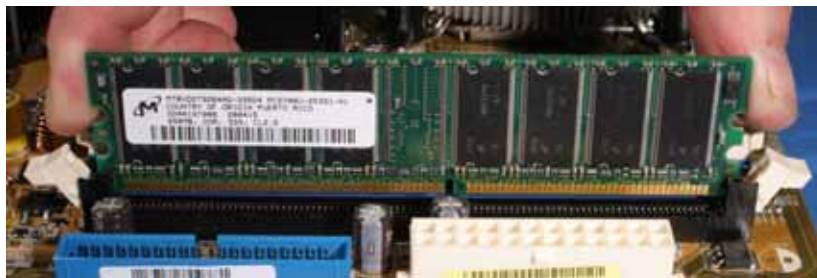
Figure 37: Remove the Module, Touching Only the Edges of the PCB
