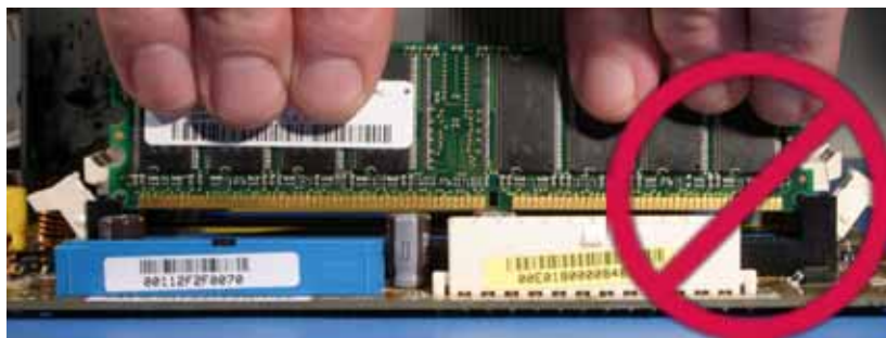
Figure 28: Never Touch the Memory Chips or Other Parts on the Module
