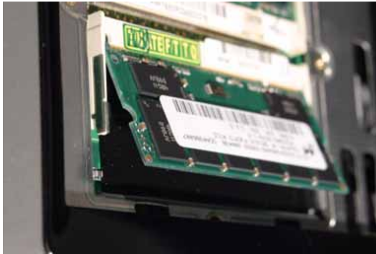
Figure 15: Step 3 – Press Down on the PCB to Set the Module into Its Final Position
