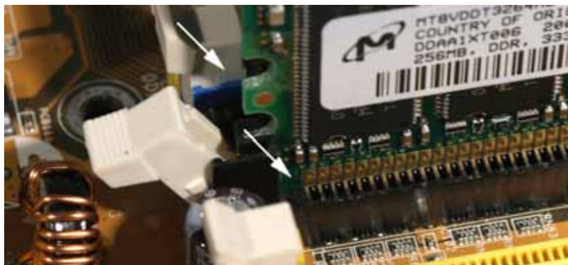
Figure 25: Step 3a – Check the Alignment of the Module and the Ejector Pins/Latches
