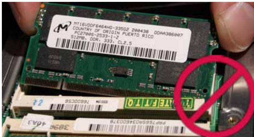
Figure 19: Never Insert Modules at an Angle or One Side at a Time
