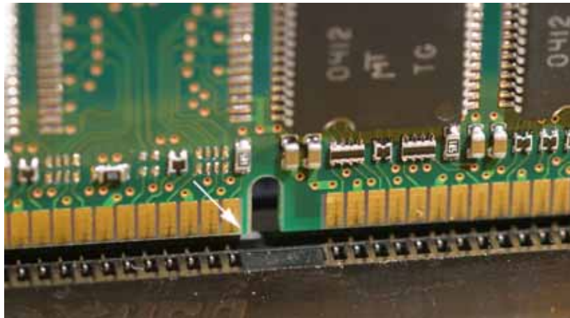
Figure 27: Step 4 – Press Down on the PCB to Set the Module into Its Final Position
