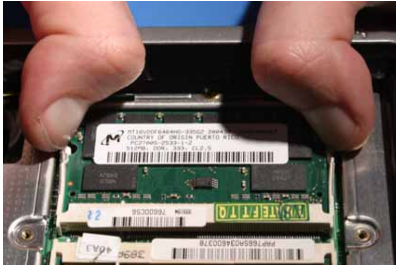
Figure 33: Remove the Module, Touching Only the Edges of the PCB
