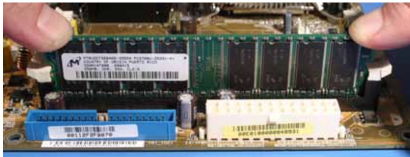
Figure 27: Step 4 – Press Down on the PCB to Set the Module into Its Final Position
