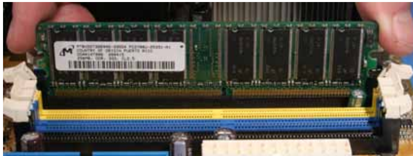
Figure 25: Step 3a – Check the Alignment of the Module and the Ejector Pins/Latches
