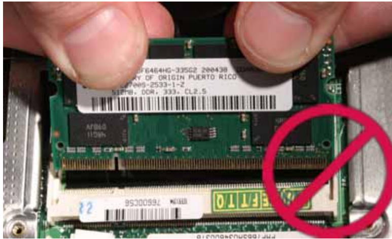
Figure 35: Never Remove the Module at an Angle
