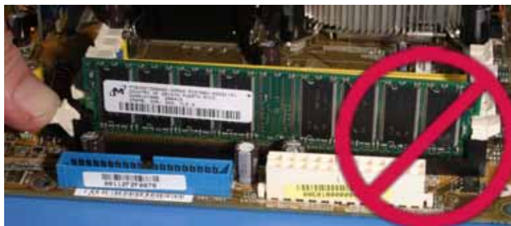
Figure 38: Never Use One Alignment Notch Alone
