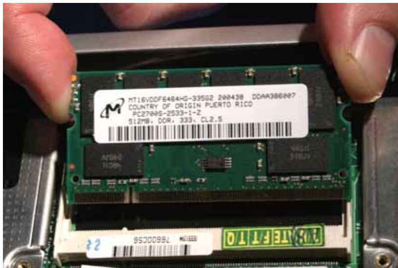
Figure 33: Remove the Module, Touching Only the Edges of the PCB
