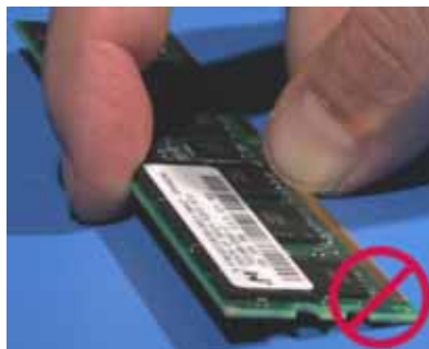
Figure 6: Never Press on the Gold Connectors and Pick Up a Module
