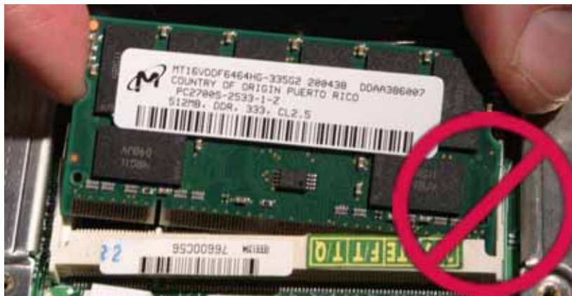
Figure 35: Never Remove the Module at an Angle
