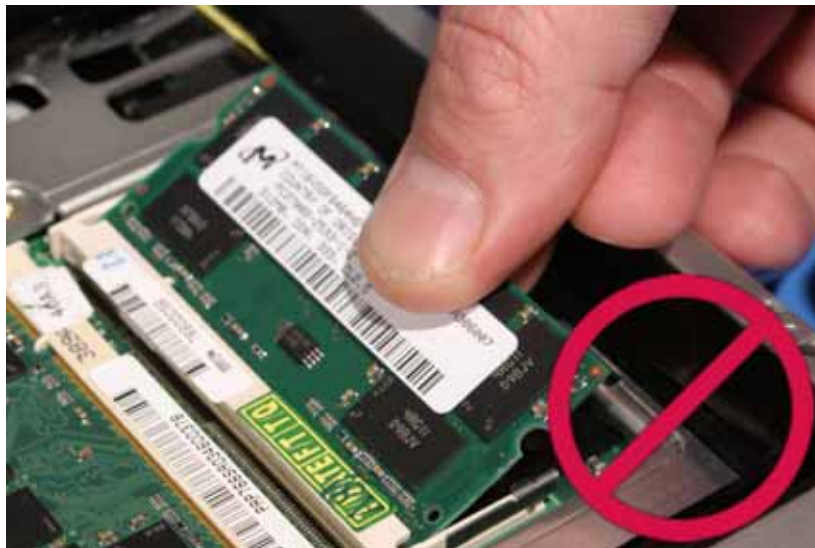
Figure 17: Never Touch the Memory Chips When Inserting the Module
