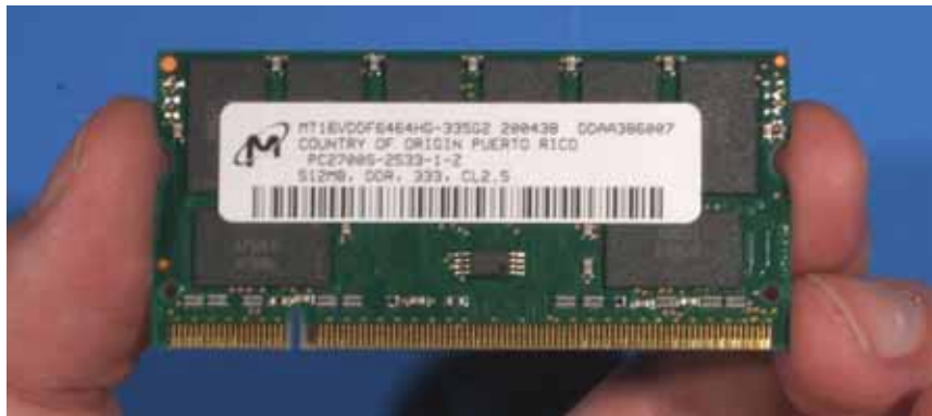
Figure 3: The Only Way to Hold a Module is by the Edges
