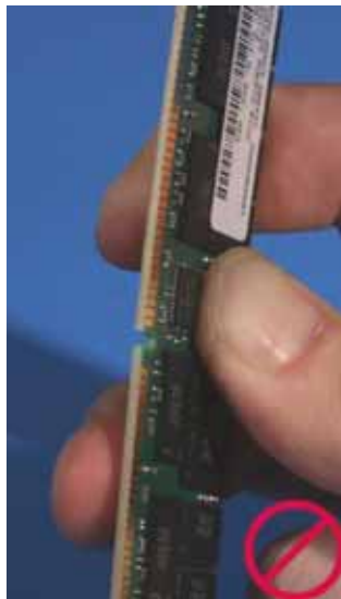
Figure 9: Never Bend or Twist a Module
