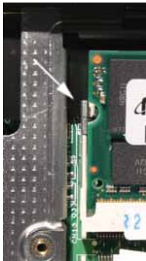
Figure 13: Step 2a – Visually Inspect the Module Alignment in the Socket
