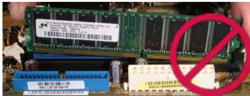
Figure 40: Never Remove the Module at an Angle
