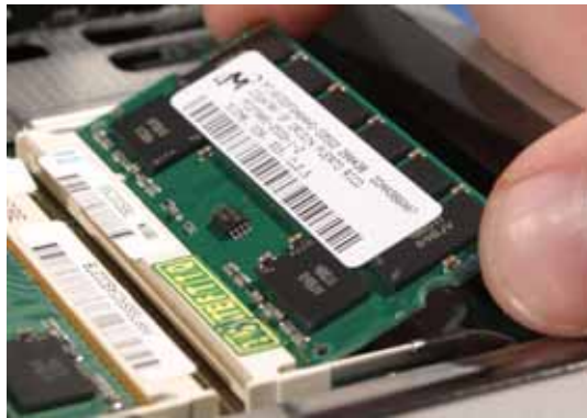
Figure 13: Step 2a – Visually Inspect the Module Alignment in the Socket
