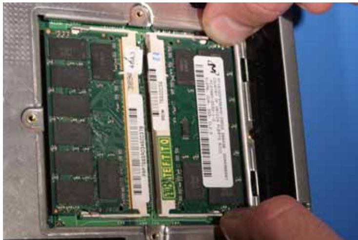
Figure 15: Step 3 – Press Down on the PCB to Set the Module into Its Final Position
