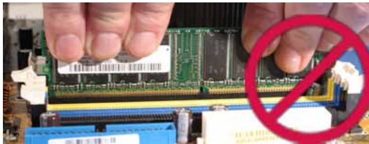
Figure 40: Never Remove the Module at an Angle
