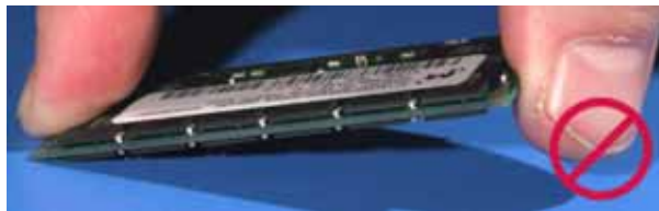
Figure 8: Never Hold a Module Using Three Points of Pressure
